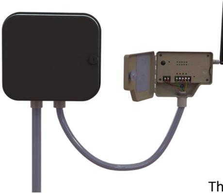
Install color-coded wire between a new or existing irrigation controller. Power the Transmitter™ from the controller's 24 VAC auxiliary power output, typically used for rain sensors or remotes
